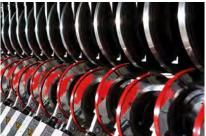
Due to the simultaneous computer controlled knife positioning all knives are adjusted at the same time with high precision. Individual knives can be adjusted automatically and manually. The intuitive touchscreen handling supports operators, enabling them to do any change of slit widths in an error-free, safe, precise and quick way. The adjustment time required will be less than 15 seconds, independent of the number of knives in operation. Inline slitting is possible with SIMU-FLASH.
