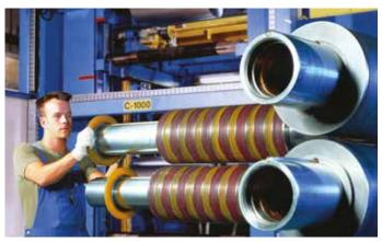
To optimise cutting production and minimise set-up time of knife shaft systems, a new computer program is available to DIENES customers. After setting a predetermined cutting plan, the program accurately defines the proper sequence for mounting cutting tools. The results are cost savings when minimum time is required to assemble tooling and test cuts during set-up are not required.
