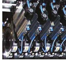
Independent of the cutting stroke and effects of heat, the DIENES pneumatic knife holders offer precise control of the important geometric slitting relationships needed for properly slit aluminium foils. Zero clearance, pre-loaded, caged linear ball bearings support both vertical and horizontal action of the knife holders.
